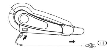
3.) Insert the plug into any convenient 120V 60Hz AC outlet.
